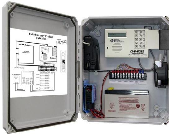
CVD-2025 is a completely self-contained, weatherproof, four-channel monitoring system and cellular automatic voice dialer. Trigger event are announced via recorded voice message delivered by the cell phone when the call is answered. Representing an exciting new level of achievement, the CVD-2025 combines technologically advanced features, ease of programming and reliable operation in a compact, unobtrusive dialer completely compatible with any security alarm system.
