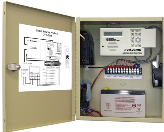
CVD-2000 is a completely self-contained, four-channel monitoring system and cellular automatic voice dialer. Trigger events are announced via recorded voice message delivered by the cell phone when the call is answered.
